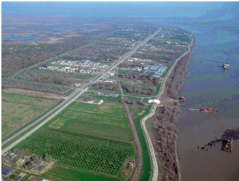
Sediment is used from the Mississippi River to rebuild wetlands in a new location. The red boat near the levee is pumping sediment to the fragile wetlands in top left of the image. The sediment is then used to rebuild marsh that had turned to open water, creating new wetlands.
