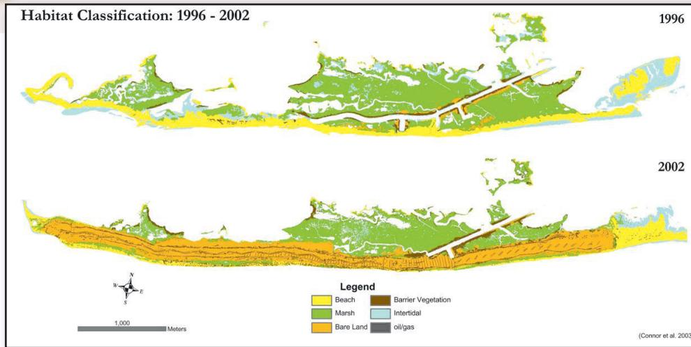
**Figure 1:** Habitat classification maps showing Trinity Island before and after the restoration project was completed. The “bare land” area on the bottom section of the map is the sediment that was pumped onto the island. done by CWPPRA, the Coastal Wetlands Planing, Protection and Restoration Act.
