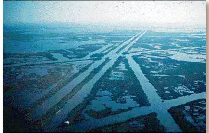
Fragile wetlands are readily damaged, directly and indirectly, by canals dredged for navigation and energy exploration. (Photo credit: USGS)
